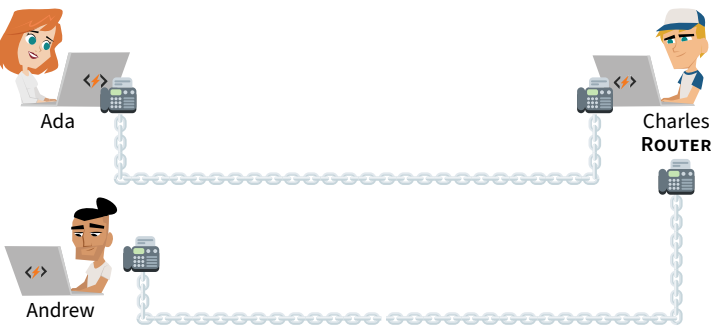
Figure 1.8 In this small LAN, Ada and Andrew can send messages to each other through their router Charles.
