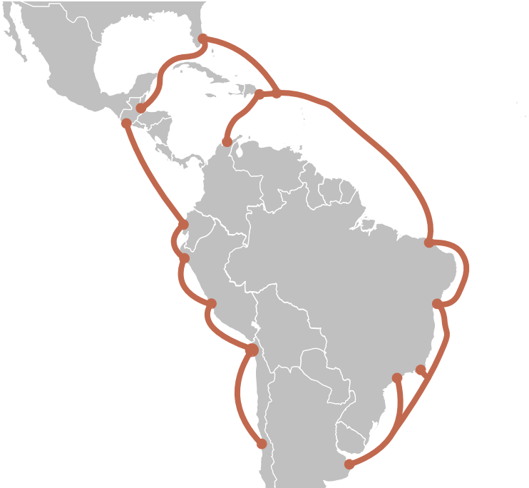
Figure 1.10 The SAM-1 system links routers in 16 cities from 11 different countries, using over 15 thousand miles of underwater cables.
